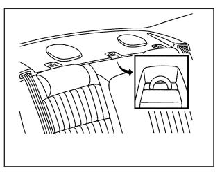
Your vehicle has top strap anchors already installed for the rear seating positions. You will find them behind the rear seat on the filler panel.
